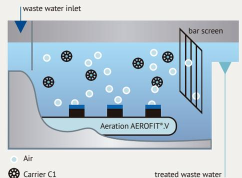
Lastly, a well-proven **restraint grid system** secures the carriers within the treatment vessel, thereby ensuring that the biofilm stays in the vessel. This restraint system is designed so that it will not clog during long-term operation.
